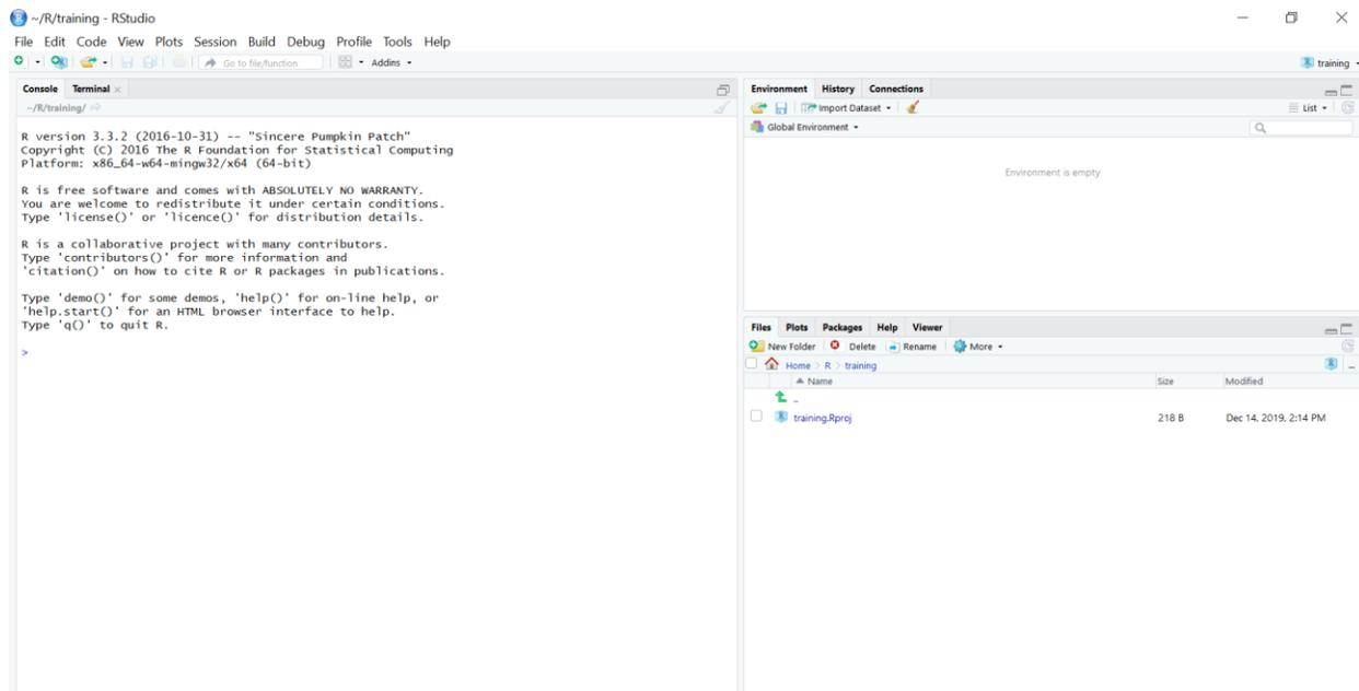
The command line environment is on the left. Images when we construct them will appear on the bottom right. As we add variables, they will appear in the list at the top right (name, dimensions and samples will display, which is useful for checking that you didn't skip entries when entering data by hand).
